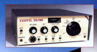
G4SLU Builds The Yeovil 3.5 And 14MHz HF Transceiver
