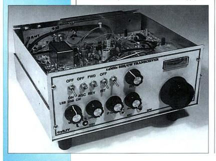
One of the prototype PW Jubilee 14MHz transceivers designed and built by G3RJV.
