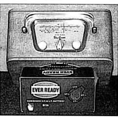
Fig. 6: The Ever Ready Sky Queen portable valved receiver, which utilised 90V h.t. valves and a 1.5V filament supply, with its associated battery (see text).
